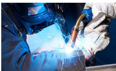
Weld on of a damaged tool (MAG welding process)
