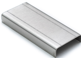
Bending result without protective film
